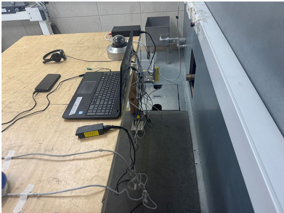
<Conducted Emissions at Telecommunication Ports - Rear>
