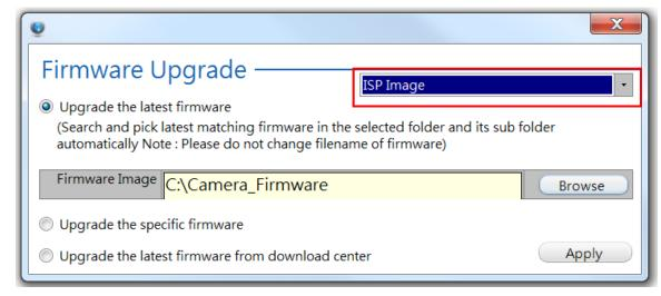
The device needs 7 minutes for ISP upgrading, and it will reboot automatically and show return message "Success" after the image upload completes.
