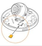
Attach the main body to the mount bracket by tightening the lock screw using the six-angle wrench. To install the camera's SD Card, locate the SD card slot in the back of the camera module. Insert a Class 10 SD card into the SD card slot by pressing the SD card slot. To remove the SD Card, press the card inward to release from the card slot.
