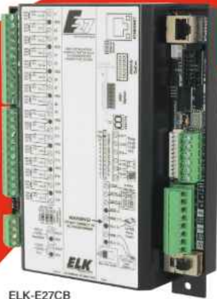
ELK-E27CB E27 Alarm Engine Control Board
