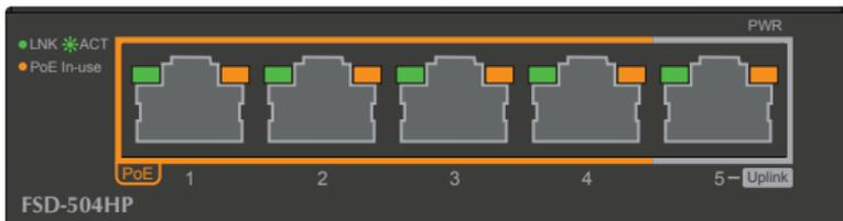
**Figure 3-1:** FSD-504HP Front Panel
