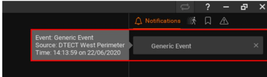
*Engineers Note: If you are unable to receive events on WAVE, check and verify all network settings including IP scheme, port & credentials. Double check sources, captions and descriptions in both GJD product and WAVE to ensure they match 100%.*
