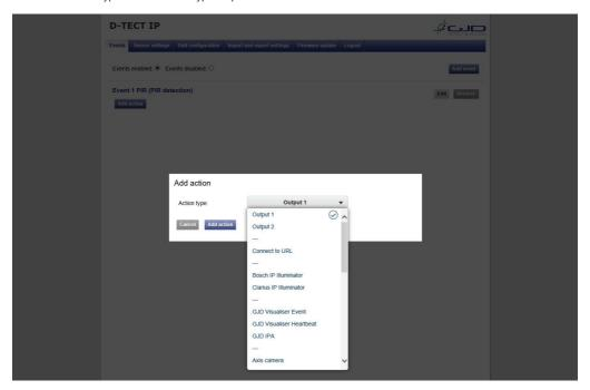
Connect to URL Connect to URL is used to create any type of network alarm. This allows one URL
