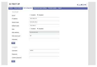
3. Enter desired settings and press the save button. Remember to reload the page with the new IP address if changed.
