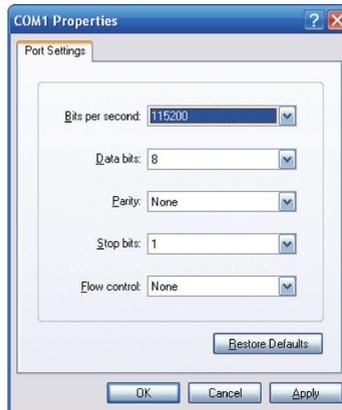
**Figure 3-2:** COM Port Configuration
