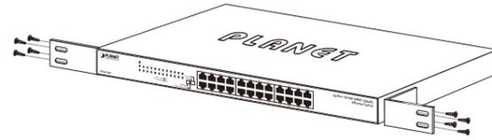
Figure 5: Attaching the brackets to the Gigabit Ethernet Switch
