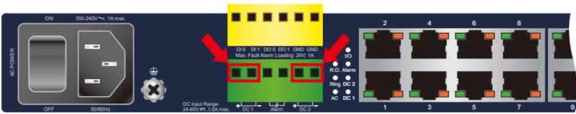
**Figure 3-2:** 6-contact Terminal Block Connector
