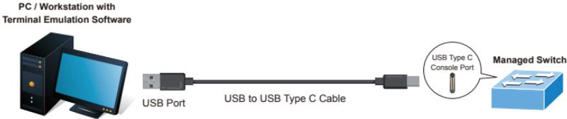
**Figure 4-1:** Industrial Managed Switch Console Connectivity
