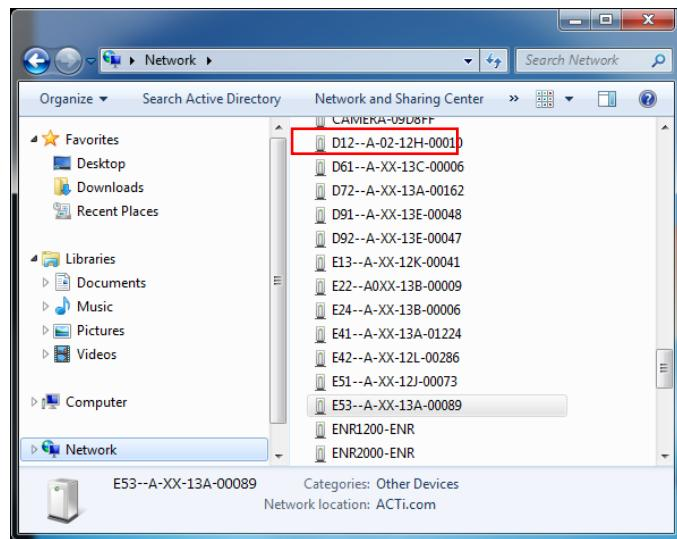
By double-clicking the mouse button on the camera model, it is possible to automatically launch the default browser of the PC with the IP address of the target camera filled in the address bar of the browser already.
