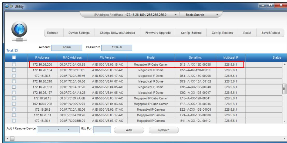
You can quickly see the camera model in the list. Click on the IP address to automatically launch the default browser of the PC with the IP address of the target camera filled in the address bar of the browser already.
