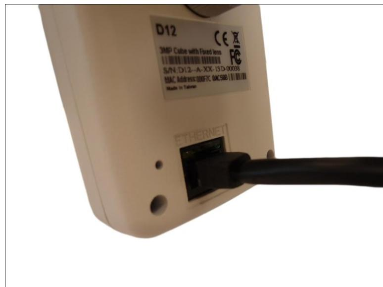
2. Connect the other end of the Ethernet cable to the PoE injector / switch.
