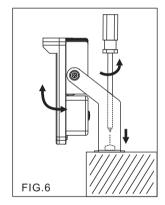
5. Adjust the vertical alignment by loosening the side bolts(one on each side of the main body) to maximize the results.
