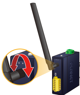
Figure 3: Connecting LoRa Antenna
