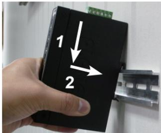
**Step 2:** Get the lower DIN-rail bracket snapped into the track.
