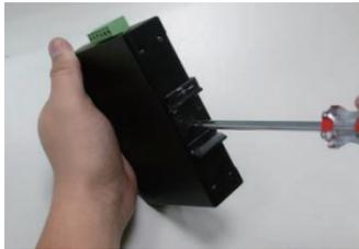
**Step 2:** Place the wall-mount plate on the rear panel of the Industrial Ethernet Extender.
