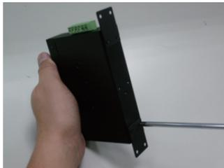
**Step 4:** Use the hook holes at the corners of the wall-mount plate to hang the Industrial Ethernet Extender on the wall.
