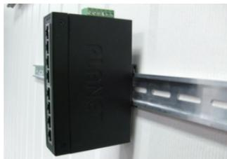
**Step 3:** Reverse the procedure to remove the Industrial Ethernet Extender from the track.
