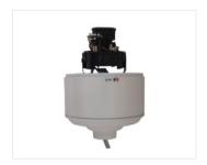
14. Mount the camera onto the mount kit using the mount kit screws (with camera o-rings) and seal the screws with silicone to protect it from water leak.
