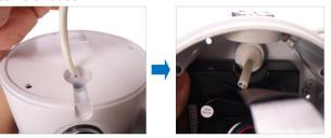
12. Once the cable length is determined (able to reach camera Ethernet port), seal the bottom cable hole with silicone to protect it from water leak.
