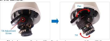
**Note:** Loosen the two tilt adjustment screws and then tilt the camera to desired angle. Tighten the tilt adjustment screws to fix the lens position.
