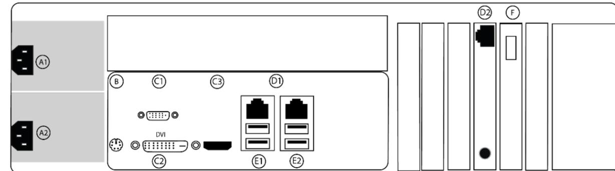
Figure 1. 2U S-Series Enterprise System back panel
