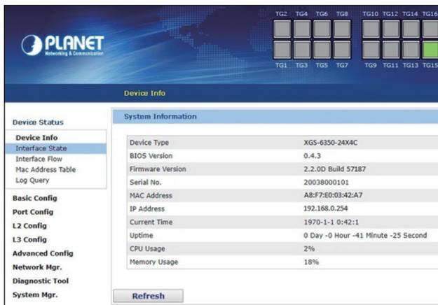
Figure 5-3 Web Main Screen of Managed Switch
