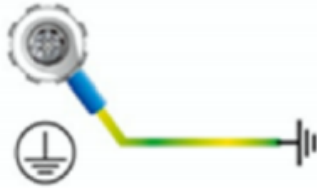
Figure 1: Socket-outlet protective earthing connection
