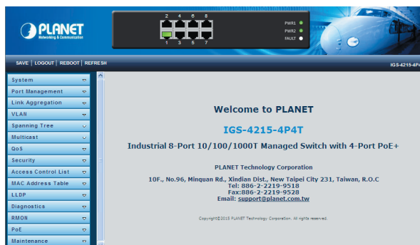
Figure 8-3: Web Main Screen of Industrial Managed Switch
