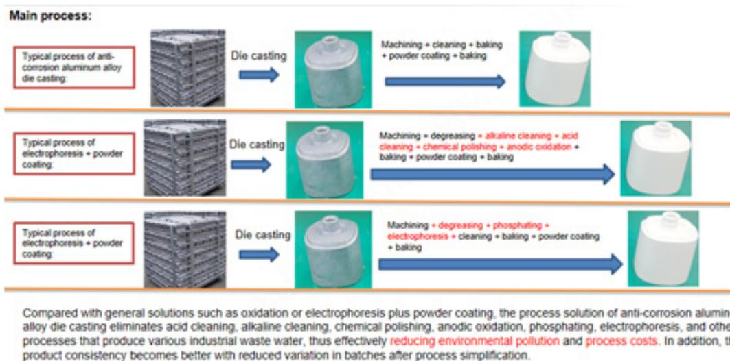
Figure 3.2 Comparison of three different corrosion-resistant solutions
