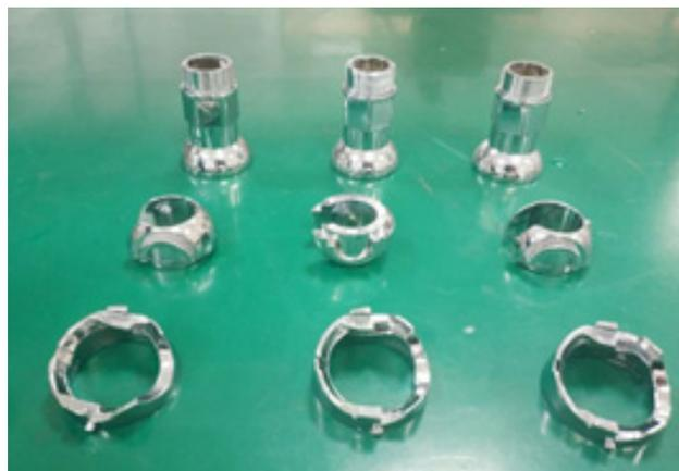
Figure 3.6 Samples after NEMA-4X salt spray test
