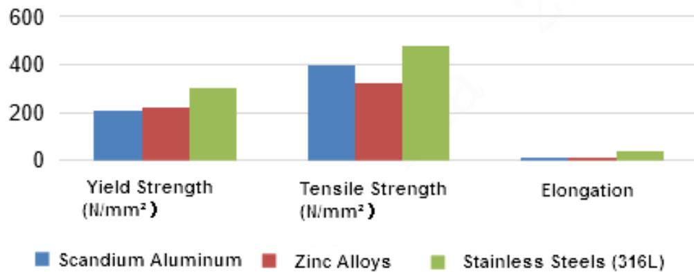
Figure 3.5 Tensile test performance parameters for different materials
