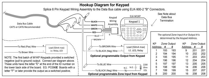
NOTE: Refer to the section 'Data Bus E.O.L. Termination' for information on multiple home run cables. NEVER SPLICE OR CONNECT WIRE WITH CONTROL POWER ON. Minimum cabling should be four conductor 22 or 24 gauge. Maximum resistance per wire is 25 Ohms. Device placement beyond 1000' is not recommended.
