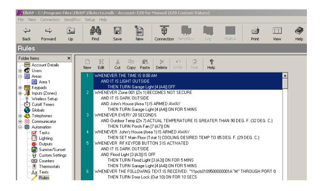
**WHENEVER -** The first element of a rule and the starting point of every rule is a triggering event. Every rule must have a triggering event in order to be started. A triggering event can be a time of day occurrence, a zone opening or closing, the security system going from armed to disarmed, a light changing from on to off, or literally hundreds of other events. Below are some examples of WHENEVER elements:
