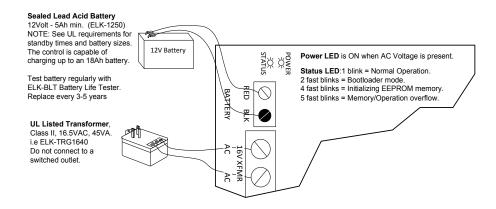
Connect the transformer to the AC Terminals using 16 to 18 gauge minimum wire. Do not exceed 50 feet between the transformer and the control or run the AC power in a multiconductor with other system circuits. Leave the transformer unplugged as well as the standby battery until all other connections have been made.
