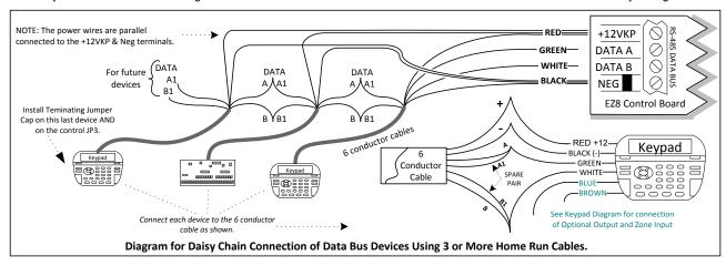
The ELK-M1DBH † Data Bus Hub accepts CAT5 or CAT6 cable with RJ45 plugs on the ends and does all the work of series connecting the DATA lines A & B. Terminate at the hub using the included RJ45 Terminating Plug in the first unused jack.
