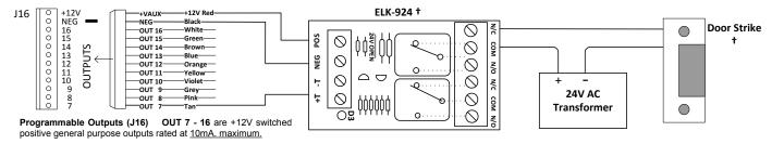
Using Output 7 (low current) with a sensitive relay to switch 24V AC to a Door Strike †
