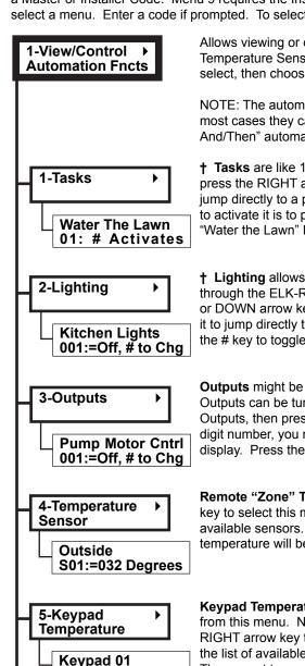
Allows viewing or controlling of the automation functions such as Tasks, Lighting, Outputs, Temperature Sensor, Keypad Temperature, and Thermostats. Press the RIGHT arrow key to select, then choose the desired function using the UP or DOWN arrow keys.
