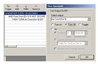
Here is an example of a rule used to turn off the air condition anytime the front door is left open by the kids. It consists of a 30 second timer for the WHENEVER trigger an AND to test the door's open/closed state, and a THEN to turn off the output that controls the air condition.
