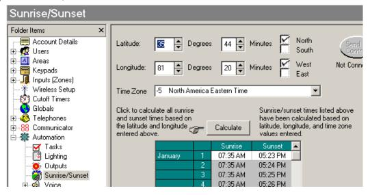
NOTE: The Time Zone automatically assumes "standard time". Therefore, the calculated times will reflect standard time. If the control is set for "Observe Daylight Savings Time" the sunrise/sunset times will be adjusted by the control accordingly.
