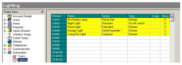
**OUTPUTS** - These can be in the form of voltage only, relays, or a combination of the two. Up to 208 outputs may be controlled. The first 32 outputs have a 16 character description, 6 word voice phrase, and the "Show" on keypad or telephone remote option. However, any output may be controlled from the keypad or telephone remote by entering its number. Outputs can be used to actuate door locks, motors, fan, pumps, etc.
