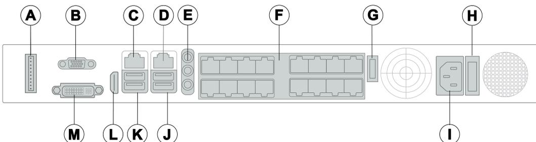
**⚠ WARNING:** Do not connect switches, routers, computers, printers, encoders, or non-camera devices to the PoE camera ports.
