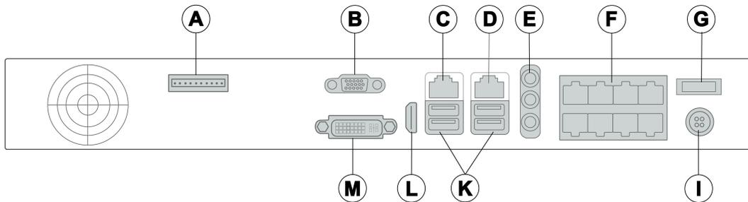
**Figure 4: Back panel connectors 16 Port G-Series PoE**
