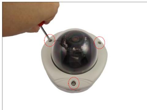
4. Carefully lift to open the dome cover and place it on the side of the camera.
