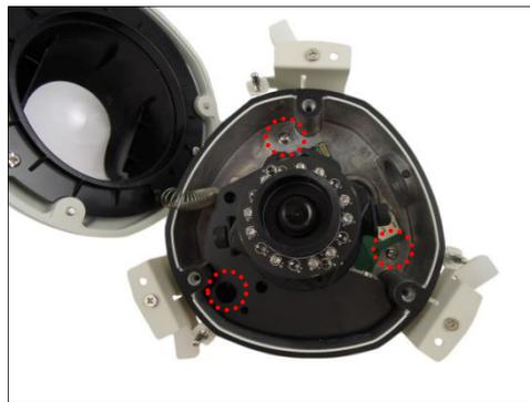
**⚠ CAUTION:** *When using electric screwdrivers*, be careful not to touch the internal camera components while attaching the screws. Since electric screwdrivers vary in sizes, speed, and force, they may bruise and damage the internal camera components.
