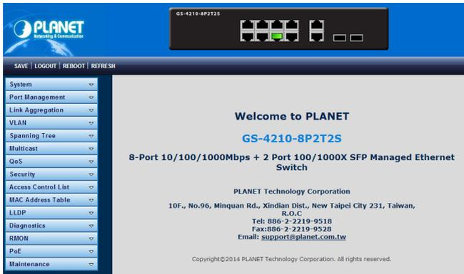
**Figure 7-3:** Web Main Screen of Managed Switch
