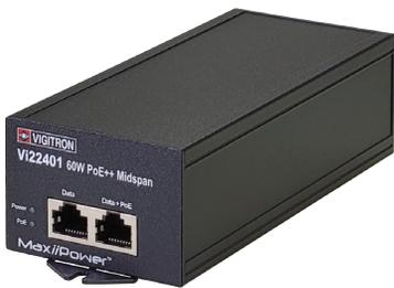
The MaxiiPower Model Vi22401 is a unique Single port PoE Midspan designed for the most demanding power applications of 10/100/1000 Base-T networks. With the ability to provide up to 60W PoE power, it is the most cost effective method for powering PTZ domes cameras with heaters and blowers. The Midspan is compliant IEEE 802.3af, IEEE 802.3at standards and 60W PoE application. Its unique control system enables it to handle both single PD and dual PD PoE devices.
