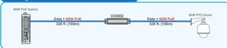
A single Vi3002 extends Ethernet and PoE from a PoE switch for total Distance of 656 ft.
